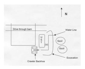
bucket into the spoil area. Without warning, the side of the excavation wall collapsed, pushing the victim against the diesel tank. 911 was called and emergency personnel arrived. Emergency personnel removed the victim from the excavation hole. The victim was taken by ambulance to a local hospital, and then air-lifted to a regional hospital where he died.
