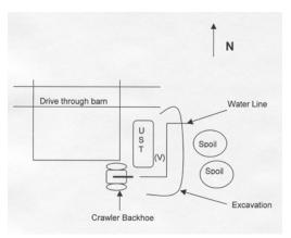
barn. He began to remove shovel loads of dirt from around the water line. One witness observed the east wall of the excavation "begin to move" and yelled to the victim "to get out of there". The wall collapsed, striking the victim from the backside, and pinning the victim, who was facing west, against the south-east corner of the tank. The soil was waist-high on the victim. The collapsed portion of the excavation wall measured approximately 1 cubic yard.
