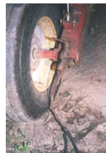
Figure 5 – Ground attached to mower
