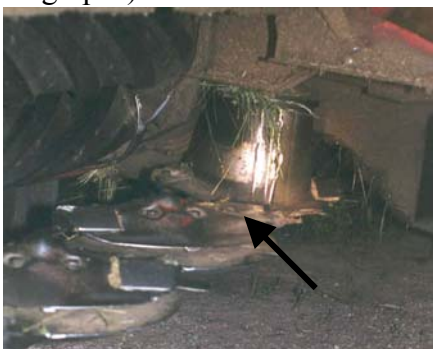
Figure 3 – Damaged Mower Disc
