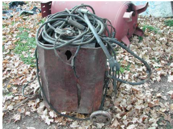
Figure 1- Overall Poor Welder Condition
