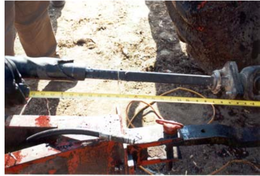
Figure 4 – Unguarded PTO shaft
