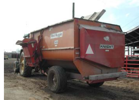
Figure 2 – Knight Brand of Auger-Mixer Wagon
