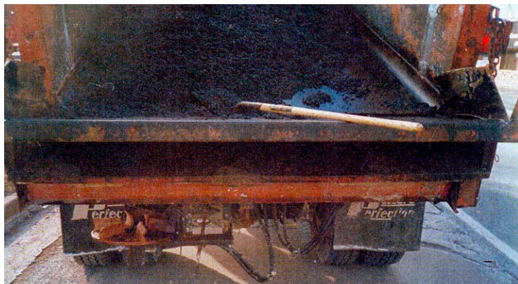
Figure 3. Cold patch in lead truck
