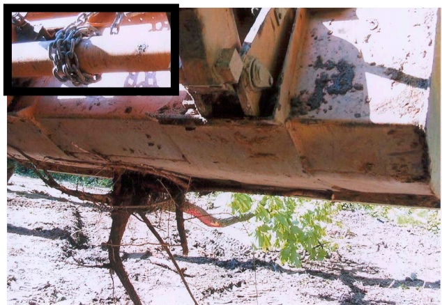
Figure 3. Chain wrapped around tree and bucket stabilizing bar
