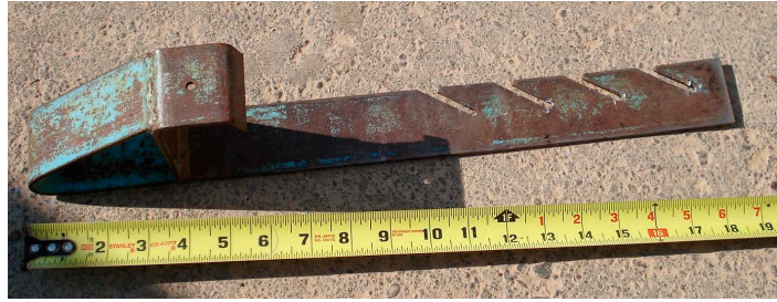
Figure 4. Roof bracket similar to type decedent installed
