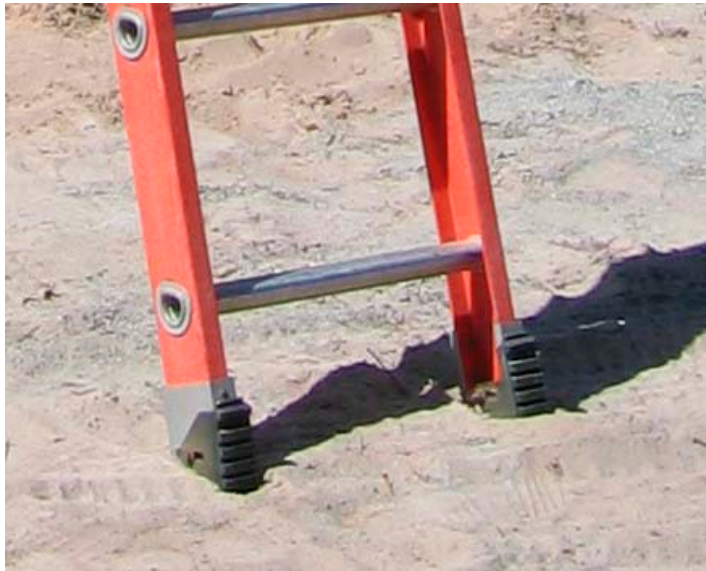
Figure 2. Ladder safety feet in the up position
