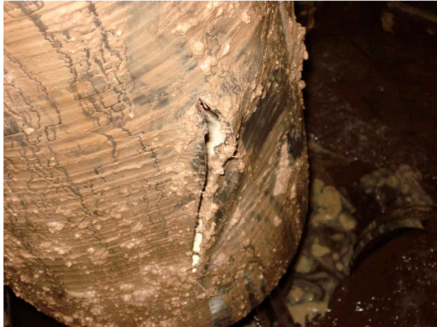
Figure 6. 16-inch cut on pipe plug
