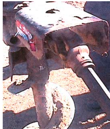
Figure 3. Auger gearbox/driveline where decedent's hood drawstring became entangled
