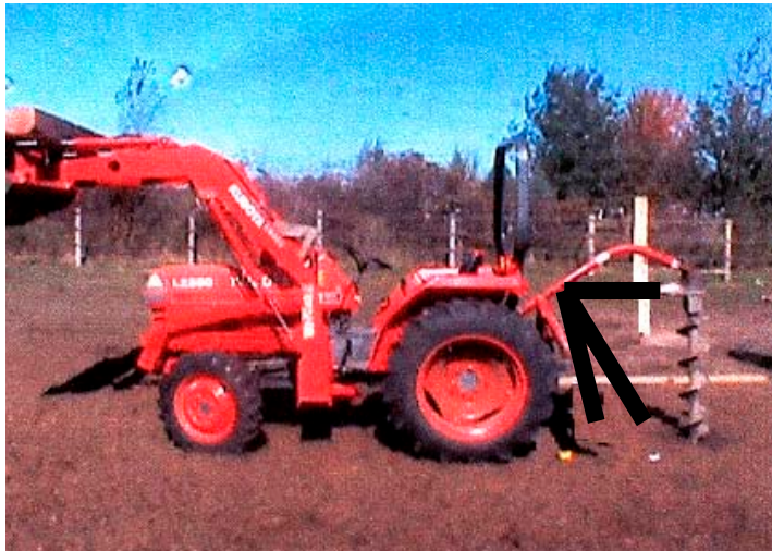
Figure 1. Tractor, posthole auger, and raised bucket arms supporting fencepost. Decedent's wrapped position around PTO shaft outlined in black
