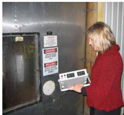
Figure 5. MIFACE researcher simulating previous CA room sampling procedure using GCS150 and sampling probe (different room)
