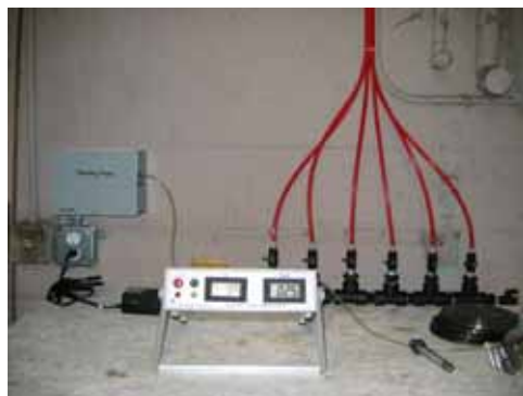
Figure 2. GCS150 and remote sampling configuration
