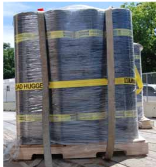
Figure 3. Shrink-wrapped roofing materials, with ratchet strap, on pallet on truck trailer
