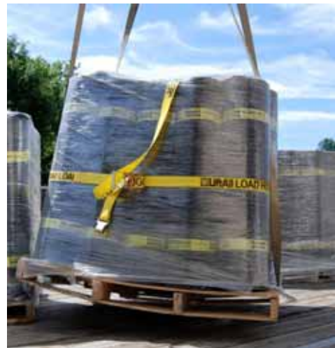
Figure 4. Police re-enactment of lift showing pallet bowing
