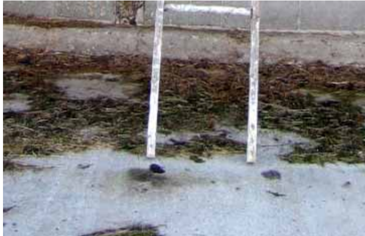
Figure 3. Ladder used by decedent with no safety feet
