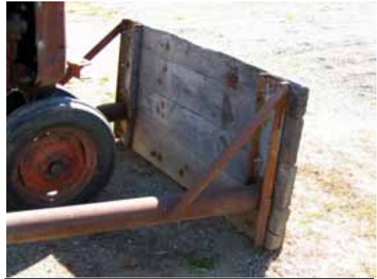
Figure 3. Close view of incident tractor showing home-made push blade attachment
