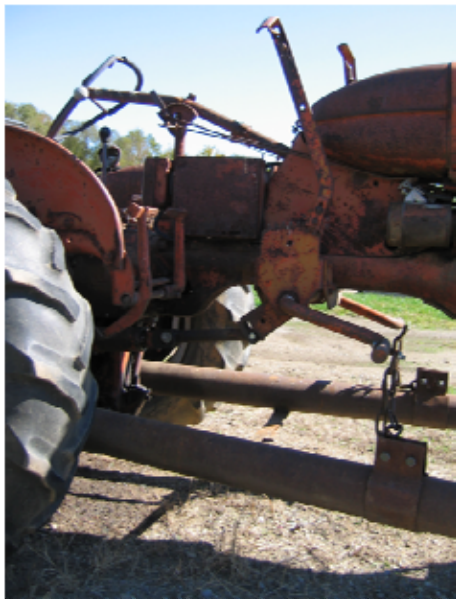
Figure 4. Attachment and hoist mechanism for raising and lowering blade
