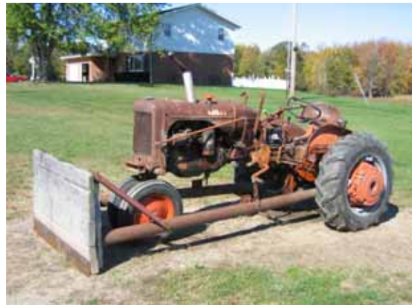
Figure 2. Incident tractor showing home-made push blade attachment
