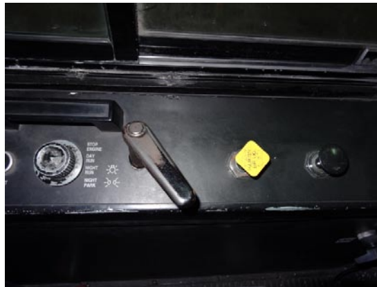
Figure 4. Unlabeled Door Controller Lever
