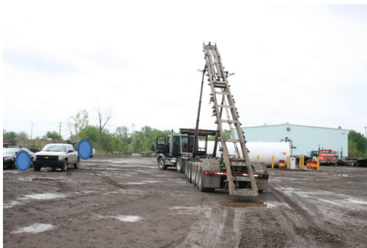
Figure 3. View of truck/trailer from near container and decedent’s location. Note that stinger is not fully on the ground.
