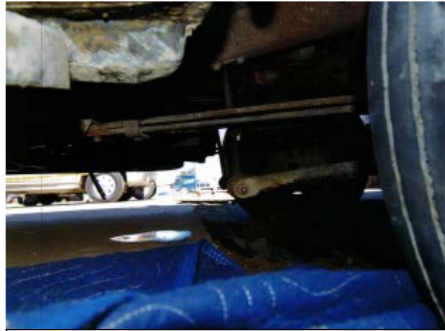
Figure 1. Picture of sway bar/linkage, passenger side, decedent's work area
