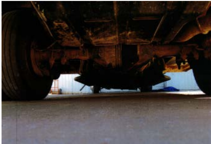
Figure 3. View of undercarriage and distance between sway bar and linkage and cement
