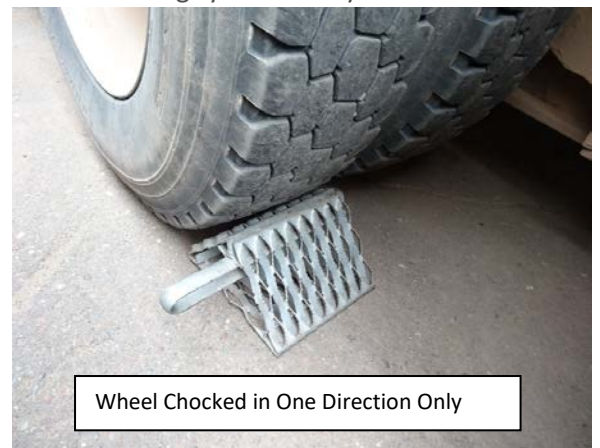
Photo 3. Example of a wheel chock in one direction
