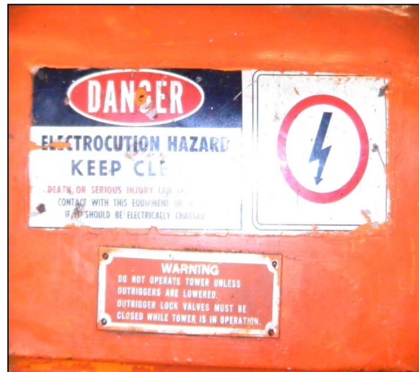
Side of a truck which served as an energized conductor that resulted in electrical burns to a tree trimming worker.
