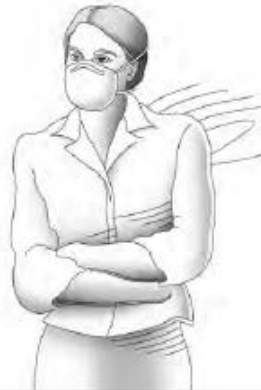
Half mask/Dust mask APF=10 Needs to be fit tested
