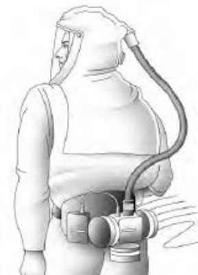
Hood Powered Air-Purifying Respirator (PAPR) APF= 25
