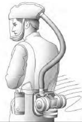
Loose-Fitting Powered Air-Purifying Respirator (PAPR) APF= 25
