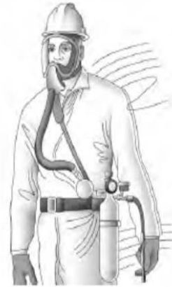
Full Facepiece Supplied-Air Respirator (SAR) with an auxiliary Escape Bottle APF=1,000 APF = 10,000 (if used in "escape" mode) Needs to be fit tested
