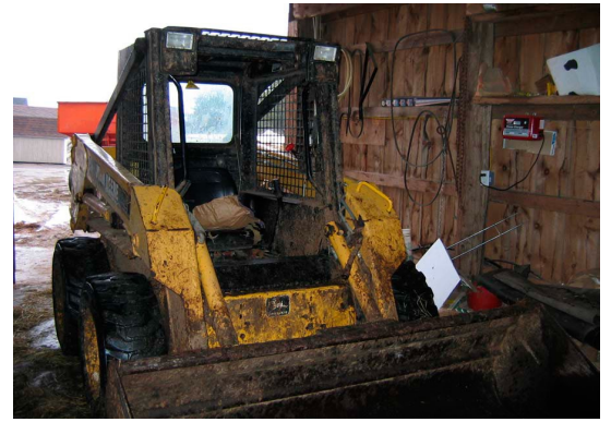
Skid steer loader with misaligned lights
