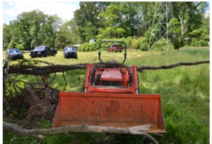
**Tractor seat struck by tree that rolled up and over the bucket**
