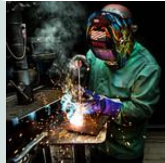
Certain hazards are common to most welding processes including burns caused by infrared and ultraviolet radiation and contact with hot metal or sparks
