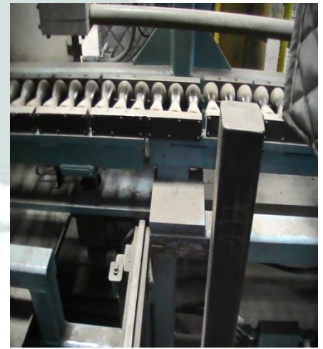
Lack of guards for pinch points is one of the causes of occupational crushing injuries
