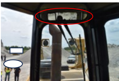
Police Photo. Rear view mirror field of view from operator seat.
