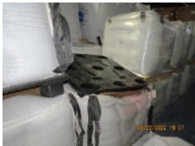
Police Photo: Collapsed lower sack causing upper sack to fall
