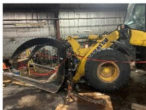
Front-end loader with log clam equipped.
