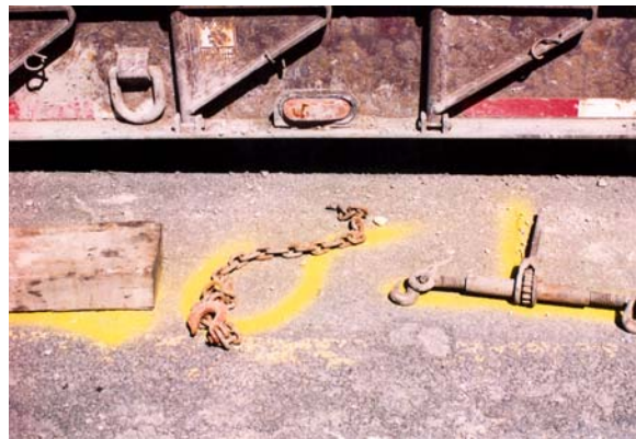
Figure 17. Oversized hook, driver's side
