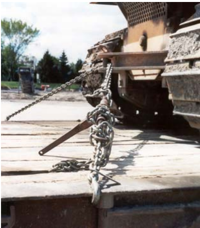
Figure 13. Improper attachment of loader to trailer bed
