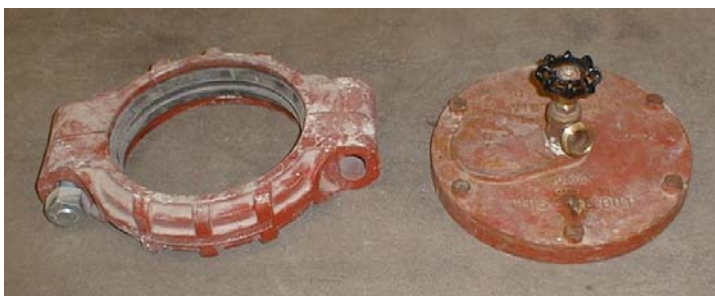
Figure 3 Coupling (left) and retrofitted grooved cap
