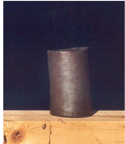
Figure 5. Side view of cylindrical steel piece used by victim as stop block
