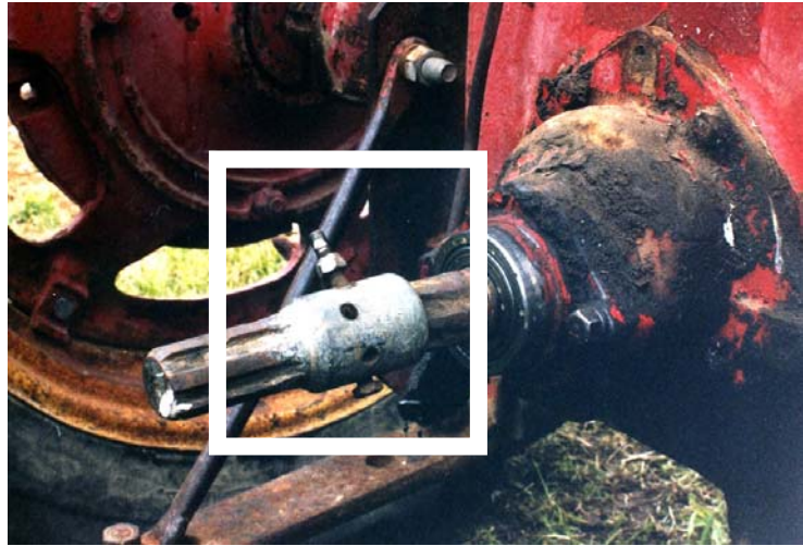
Figure 6. Unguarded PTO extension bolt
