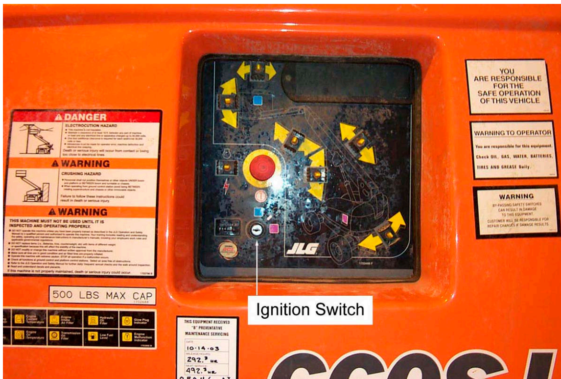
Figure 4. Ground Control Panel - Taken Immediately Following Incident Illustrating Missing Key
