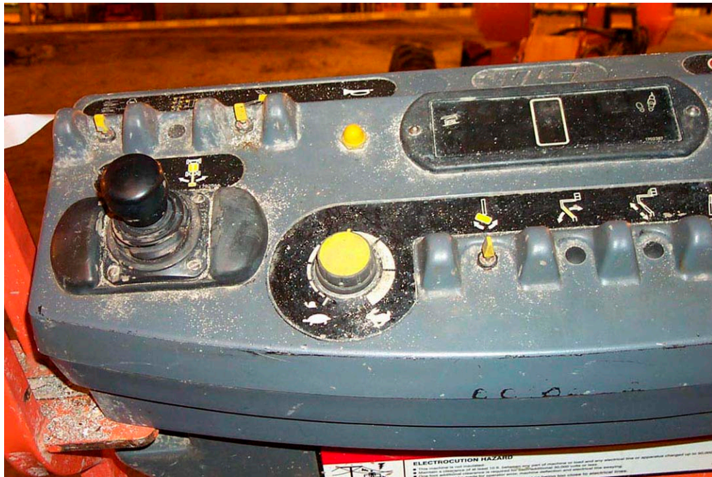
Figure 3. Basket Control Panel
