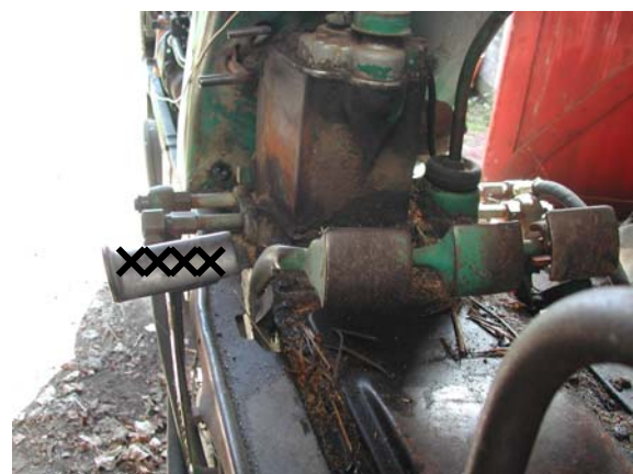
Figure 9. Crosshatch design on clutch pedal
