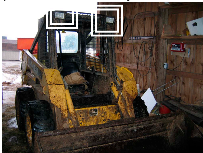
Figure 3. Non-aligned front lights on skid-steer loader
