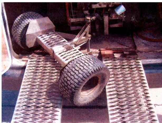
Figure 4. Position of rider platform tires outside of van
