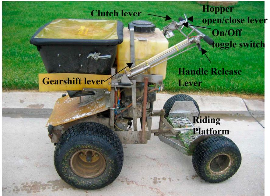
Figure 2. Ride-on spreader/sprayer
