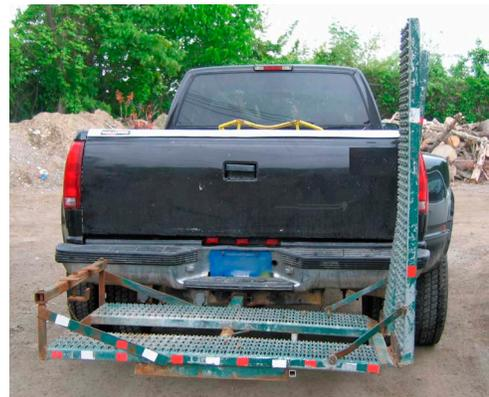
Figure 6. Basket mounted on pickup truck
