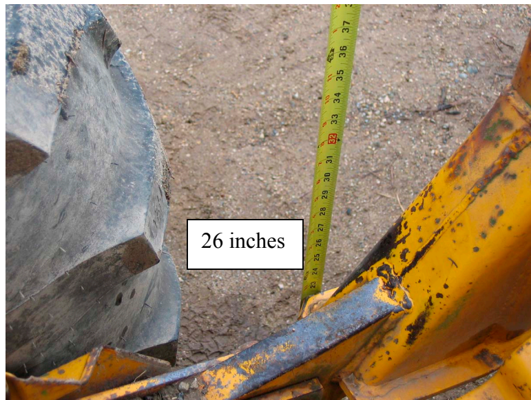
Figure 2. Height of subframe from ground
