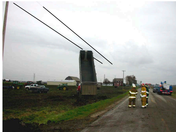
Figure 1. Extended trailer bed touching power lines (lines enhanced for clarity)
