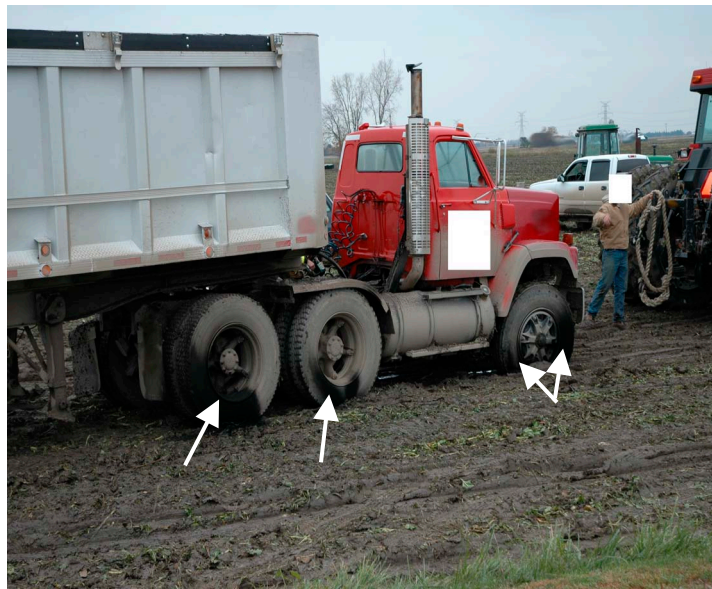
Figure 2. Evidence on the tires of electrical current seeking ground
