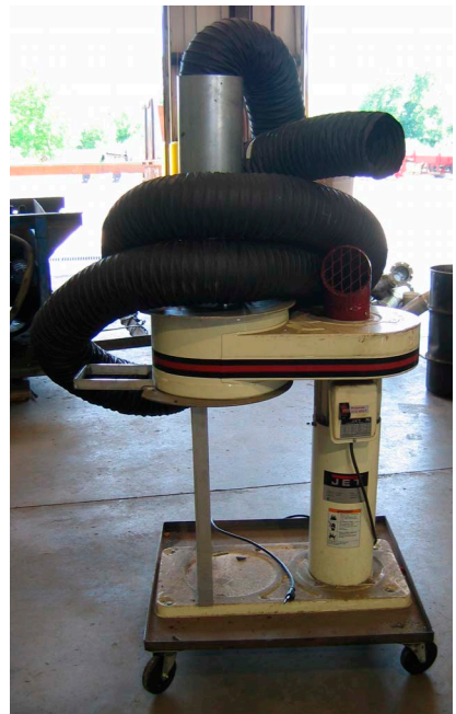
Figure 3. Example of forced air blower unit
