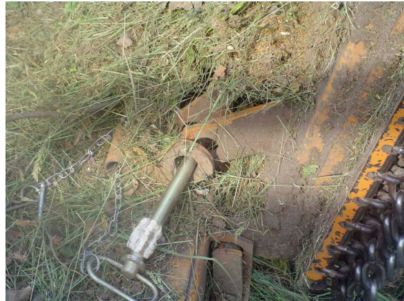
Figure 4. Bent mower locking pin
