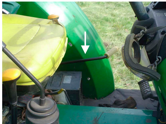
Figure 3. PTO lever engaged for mower blades to turn
