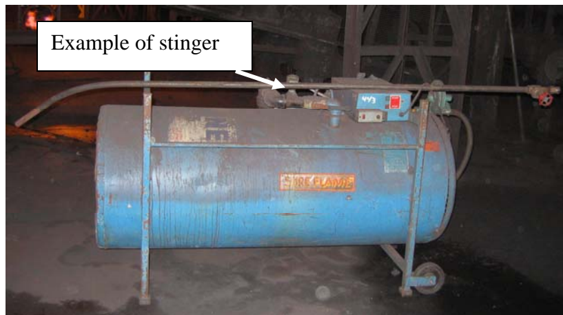
Figure 3. Tornado heater with example of stinger resting on top
