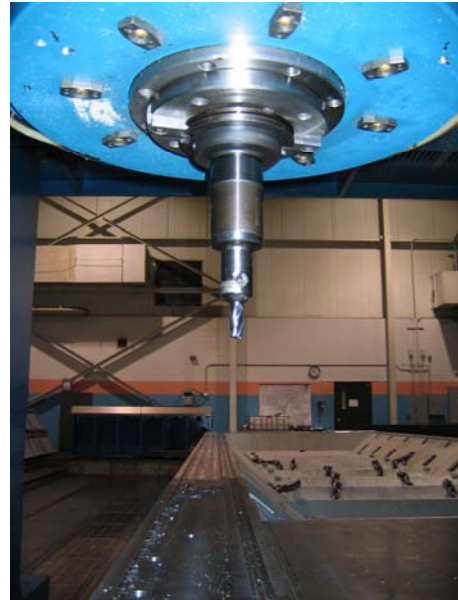
Figure 1. Cutting head of vertical gantry mill and part being machined
