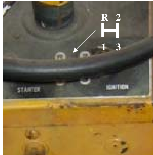
Figure 4. Gearshift pattern of tractor
