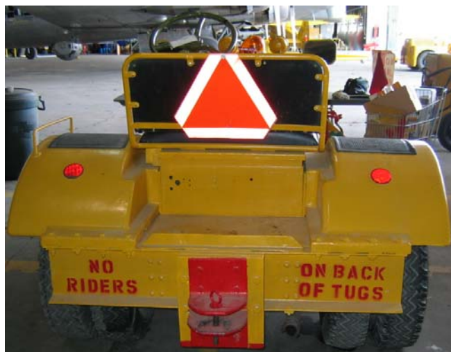
Figure 2. Back of aircraft tug showing storage area and rider warning
