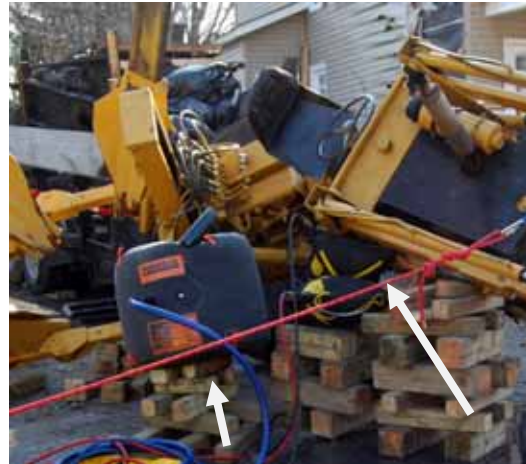
Figure 6. Lifting bags “maxed out”
