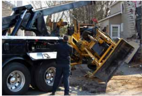
Figure 8. Use of heavy duty tow truck to upright DitchMaster
