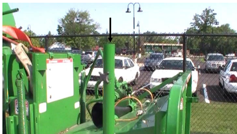
Figure 2. Arrow indicates empty push paddle holder
