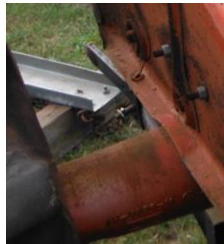
Figure 2. Attachment point of chain to wood and lift arm of three point hitch on decedent’s right side
