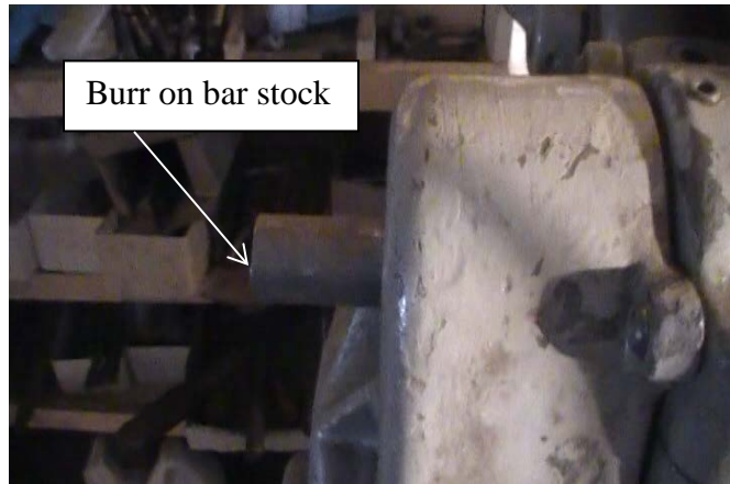
Figure 1. Burr on 1-inch diameter bar stock that caught the decedent's shirt.
