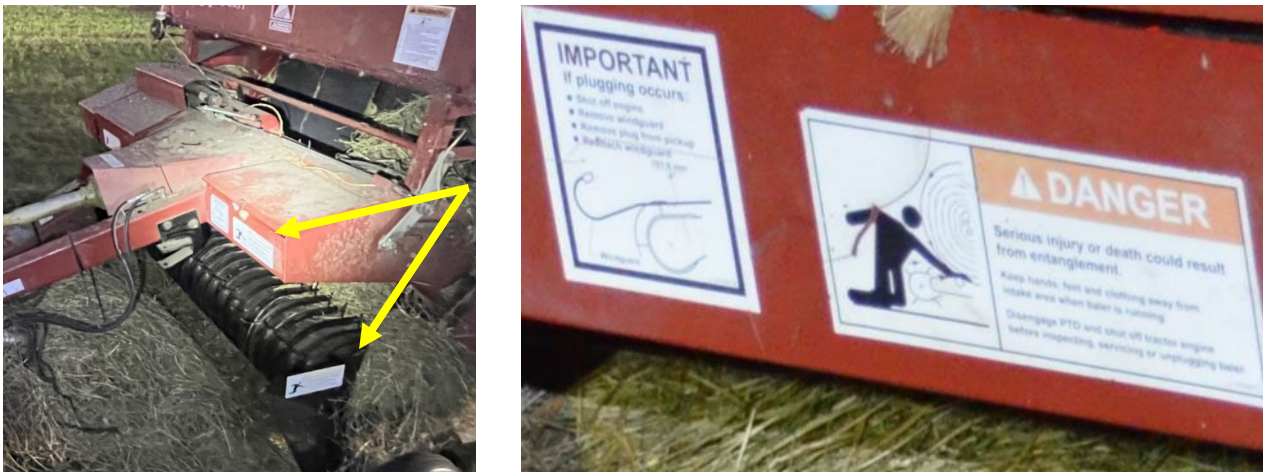
Photos 8/9: (Left) The location of the warning labels on the hay baler. (Right) An enlargement of the top warning label. (Photo source: responding police department.)
