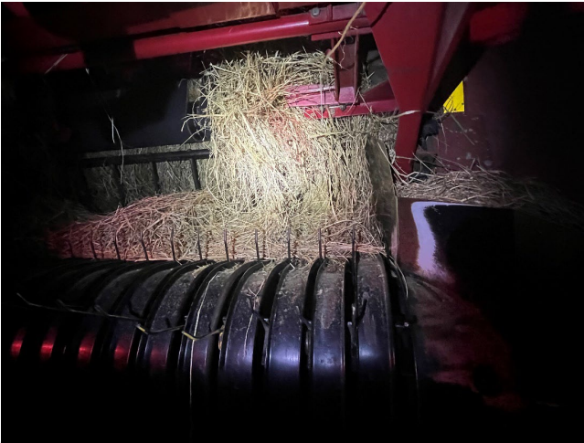
Photo 4: New Idea 4854 baler entry looking into baler pickup entry from front. (Photo source: responding police department.)
