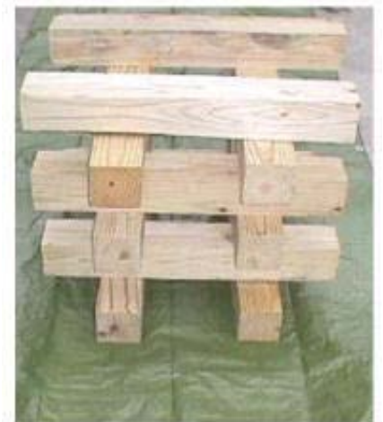
Figure 2. Example of cribbing
