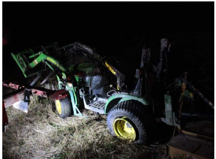
Photo 7. Condition of tractor after being removed from ditch. Note elevated bucket and flat driver's side rear tire.
