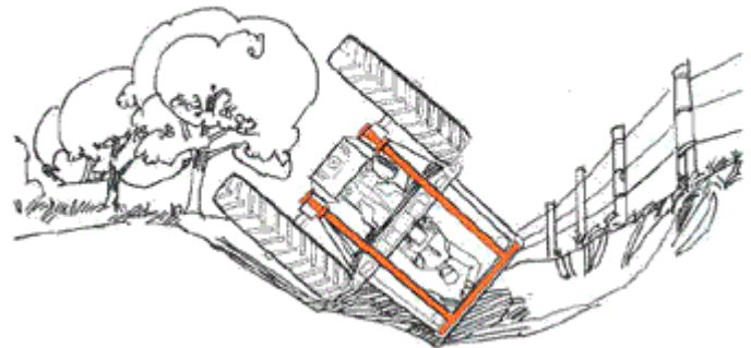
Figure 1. ROPS protecting operator in tractor overturn to side
